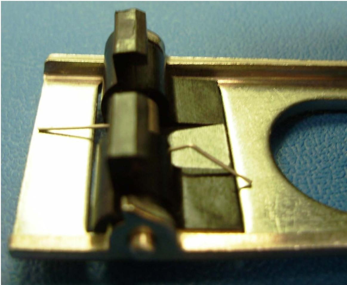
The spring end now forms a leaf spring that will contact the lid surface when closed. The height of the spring end determines the amount of deflection. The picture below shows the lid lever and latch spring just prior to being fully closed.
