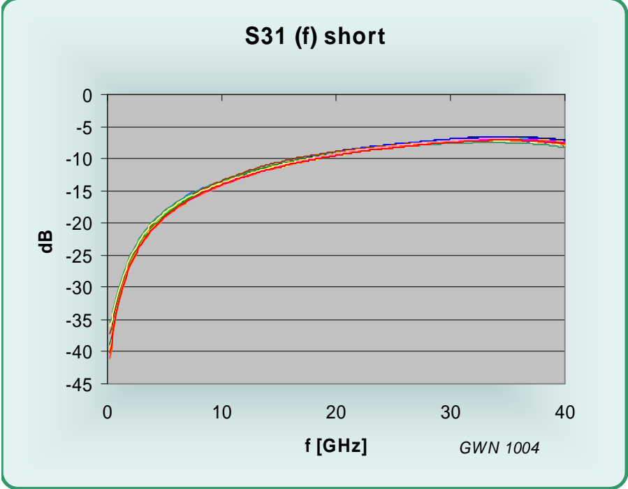
Figure 45 Short circuit crosstalk from port 1 to port 3
