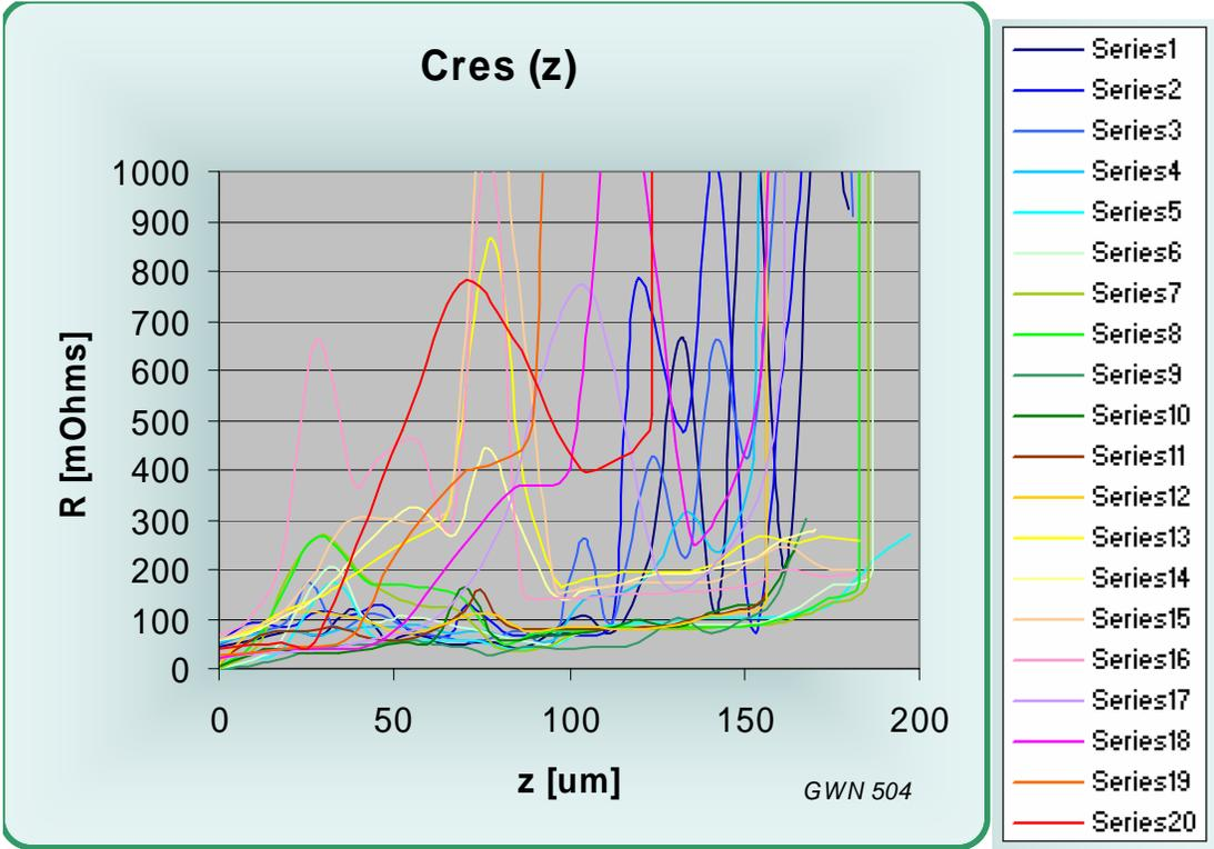
Figure 9 Contact resistance as a function of displacement
