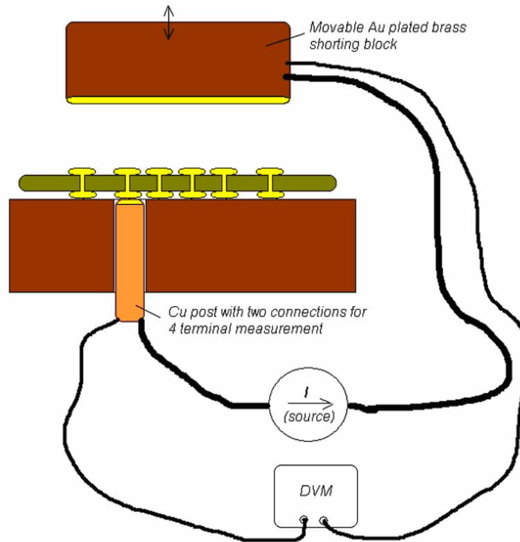
Figure 6 Test setup for 4 terminal (Kelvin) measurements
