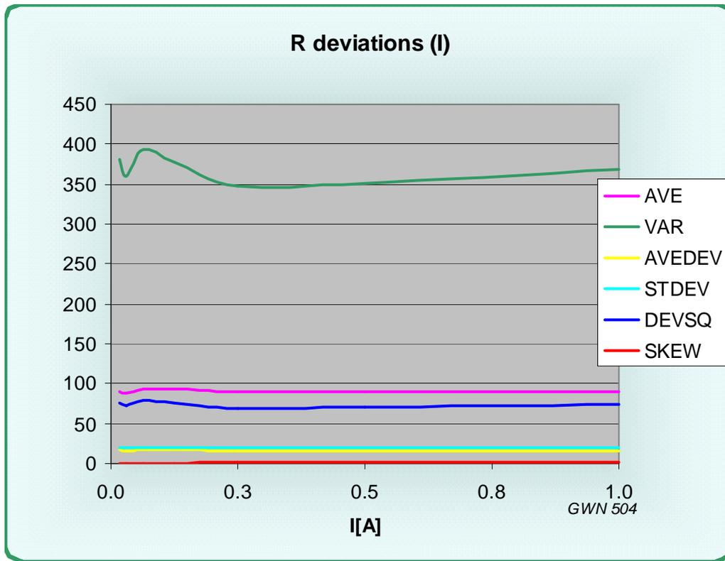
Figure 15 Deviations as a function of drive current
