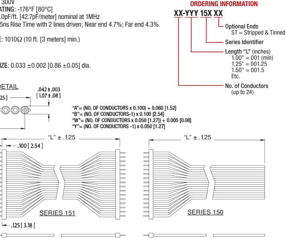
ALL DIMENSIONS: INCHES [MILLIMETERS] ALL TOLERANCES: ±0.005 [0.13] UNLESS OTHERWISE SPECIFIED CONSULT FACTORY FOR OTHER SIZES AND CONFIGURATIONS
