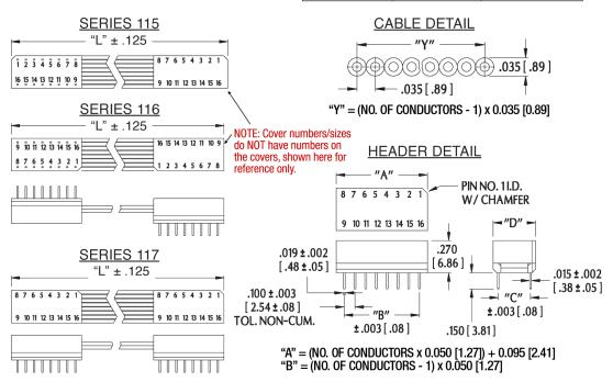
**ALL DIMENSIONS: INCHES [MILLIMETERS]** ALL TOLERANCES: ±0.005 [0.13] UNLESS OTHERWISE SPECIFIED CONSULT FACTORY FOR OTHER SIZES AND CONFIGURATIONS
