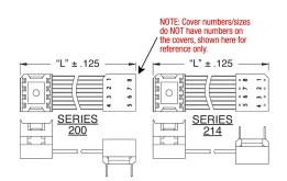
$\label{eq:approx_1} \begin{array}{l} "A" = (\text{No. of Conductors x } 0.050 \; [1.27]) + \; 0.095 \; [2.41] \\ "B" = (\text{No. of Conductors -1}) \; x \; 0.050 \; [1.27] \\ "E" = (\text{No. of Conductors +1}) \; x \; 0.050 \; [1.27] \\ "F" = (\text{No. of Conductors -1}) \; x \; 0.050 \; [1.27] \end{array}$
