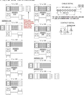
ALL DIMENSIONS: INCHES [MILLIMETERS] ALL TOLERANCES: ±0.005 [0.13] UNLESS OTHERWISE SPECIFIED CONSULT FACTORY FOR OTHER SIZES AND CONFIGURATIONS CUSTOMIZATION: ARIES SPECIALIZES IN CUSTOM DESIGN AND PRODUCTION. SPECIAL MATERIALS, PLATINGS, SIZES, AND CONFIGURATIONS CAN BE FURNISHED, DEPENDING ON QUANTITY.
