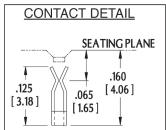
ALL DIMENSIONS: INCHES [MILLIMETERS] ALL TOLERANCES: ±0.005 [0.13] UNLESS OTHERWISE SPECIFIED FOR WIRE WRAP PINS, SEE <u>DATA SHEETS 12005</u> CONSULT FACTORY FOR OTHER SIZES AND CONFIGURATIONS CUSTOMIZATION: ARIES SPECIALIZES IN CUSTOM DESIGN AND PRODUCTION. SPECIAL MATERIALS, PLATINGS, SIZES, AND CONFIGURATIONS CAN BE FURNISHED, DEPENDING ON QUANTITY.
