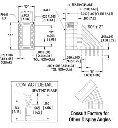
"A"= (NO. OF PINS PER ROW x 0.100 [2.54]) +0.050 [1.27] "B"= (NO. OF PINS PER ROW -1) x 0.100 [2.54]
