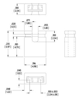
ALL DIMENSIONS: INCHES [MILLIMETERS] ALL TOLERANCES: ±0.005 [0.13] UNLESS OTHERWISE SPECIFIED CONSULT FACTORY FOR OTHER SIZES AND CONFIGURATIONS CUSTOMIZATION: ARIES SPECIALIZES IN CUSTOM DESIGN AND PRODUCTION. SPECIAL MATERIALS, PLATINGS, SIZES, AND CONFIGURATIONS CAN BE FURNISHED, DEPENDING ON QUANTITY.
